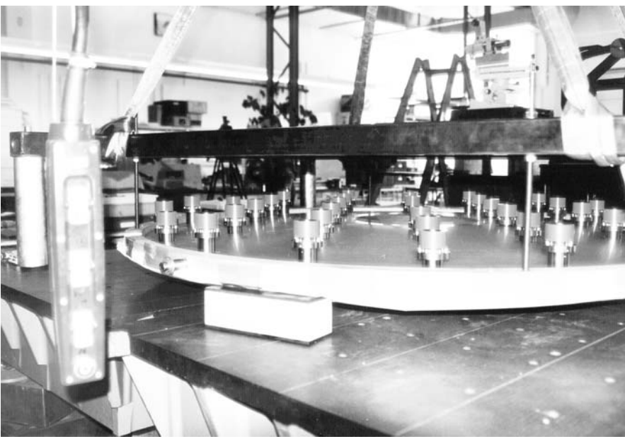
Figure 2: The raw primary with its 36 permanently fixed support units at Carl Zeiss, Jena.
