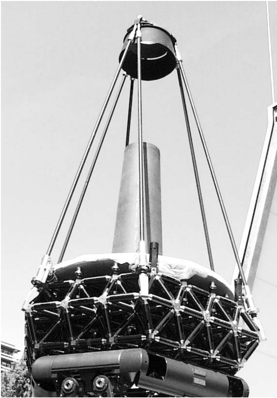
Figure 4: The Hexapod for the secondary mirror.
