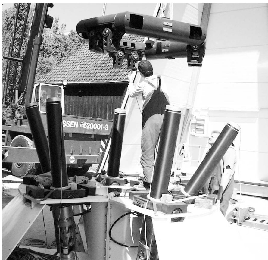
Figure 1: The length variable struts of the Hexapod mounting and the ring structure that combines the upper Cardan axes. The lower system of Cardan axes and the linear drives are also visible.
